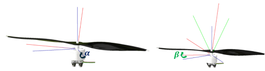
Fig. 2 \alpha and \beta angles for determining the rotors orientation
