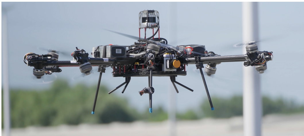
Fig. 3 Final UAV, 2nd version rotors disposition
