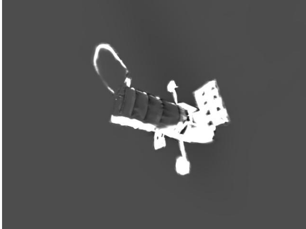
Fig. 11 After many frames, the scene gets very bright due to wrong densification settings.
