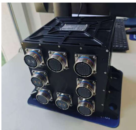
Fig.18 Flight control computer with high performance processors
