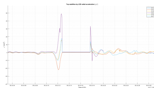
Fig. 5 LOS dynamics of the most affected satellites during parachute opening and ground touch down
